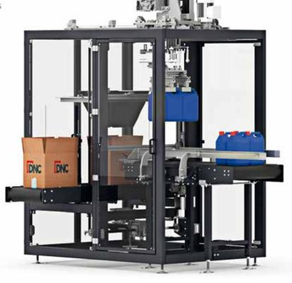
Automatic packer for rigid or semi-rigid products, adaptable to any production line. Equipped with a quick format change system to work with multiple references. The ideal solution for medium and low production lines.
